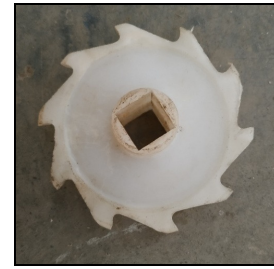
Fig. 3 : Seed metering rotor selected for soybean and cotton seed
